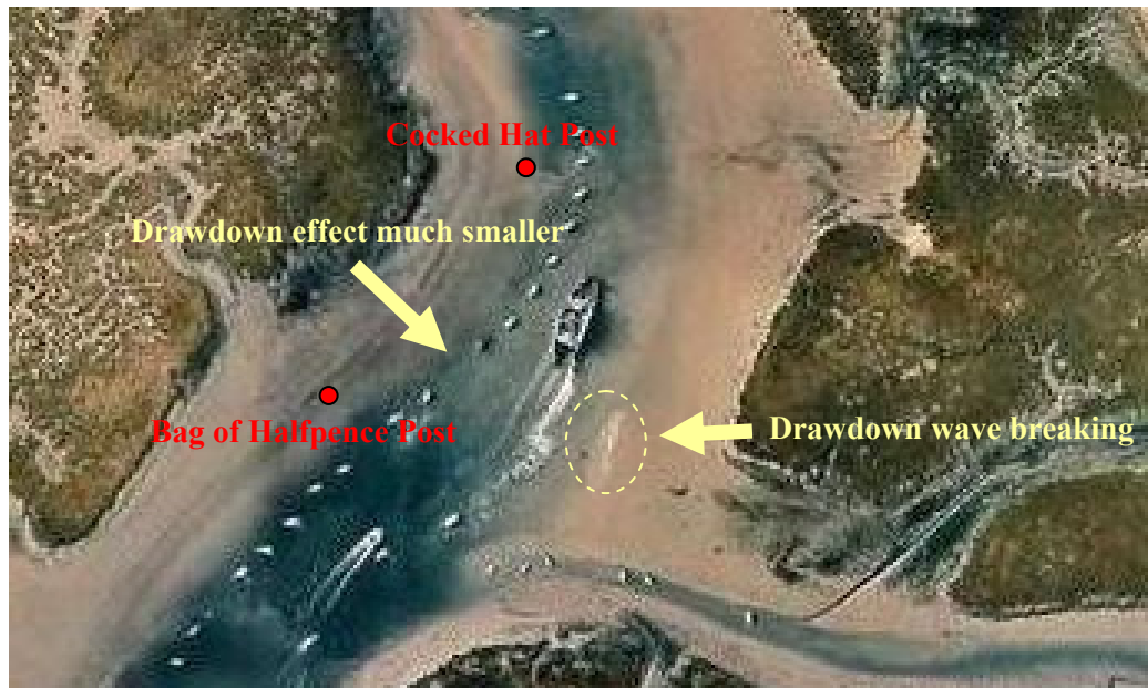
Figure 2 Aerial photograph showing effects of drawdown from inbound ferry (Photograph shown by kind permission of Lymington Harbour Commissioners)
