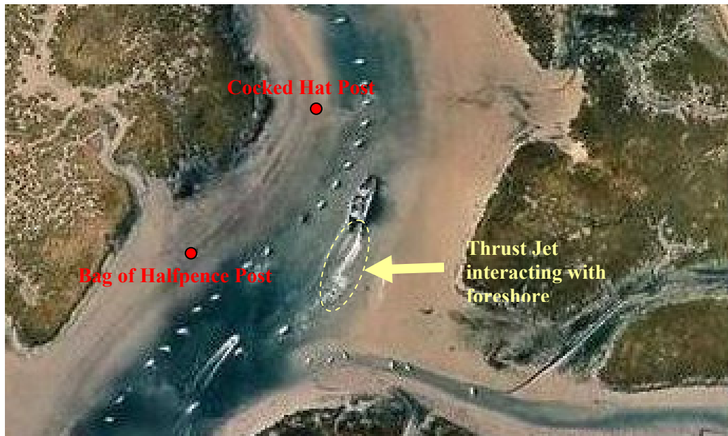
Figure 3 Aerial photograph showing C Class ferry thrust jet interacting with foreshore (Photograph shown by kind permission of Lymington Harbour Commissioners)
